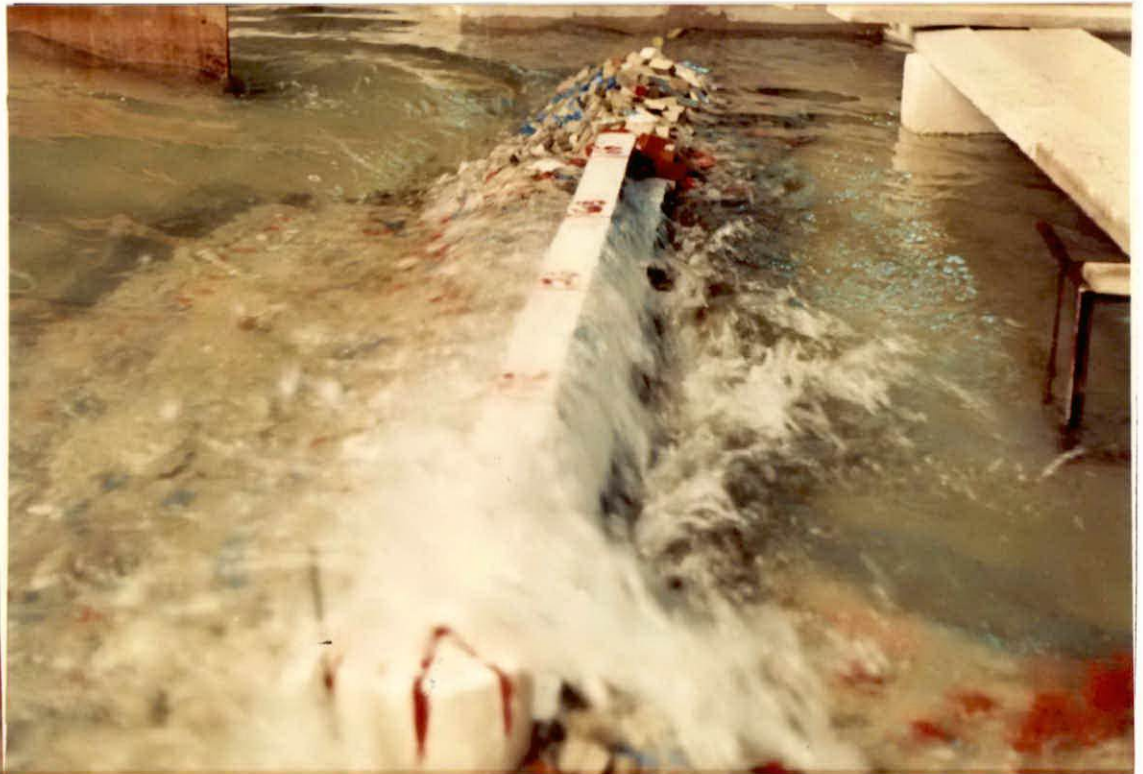
PHOTO 20 : Importance des franchissements, variante 1, direction N50° essai 9 (Hs= 9,71m, Tp=10s).
