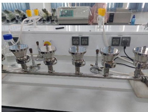
Figure 17: Rampe de filtration.
