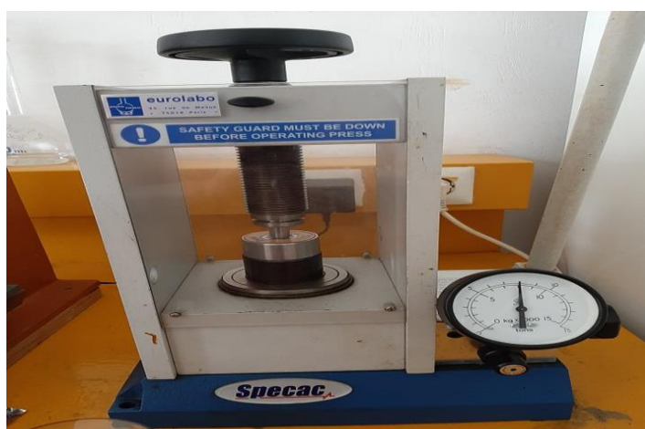
Figure II.9: Compression et formation de la pastille
