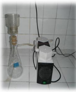
Figure 4: Pompe de filtration
