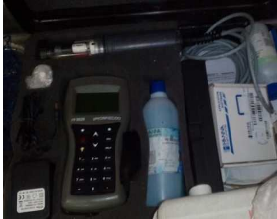
Figure III.2 : valises multi-paramètres HANNA HI9828 Ph/ORP/DO.
