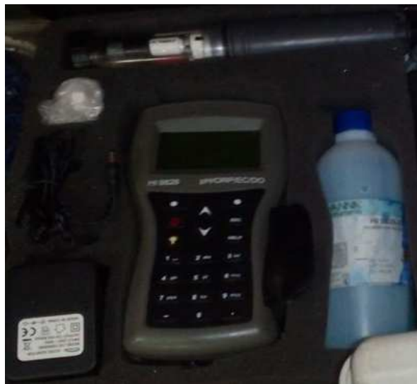
Figure III.6: valise multi-paramètre HANNA HI9828 pH /ORP/ DO.
