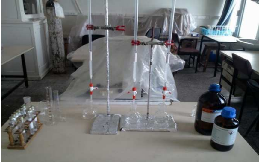
Figure 11: Les colonnes de purification
