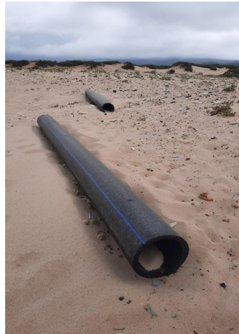
Figure 27: Tube HDPE PE100.
