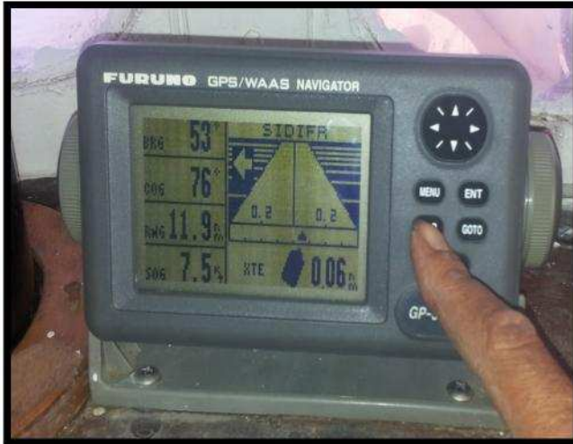
Figure 3.5 : furuno GPS/WAAS NAVIGATOR GP 32
