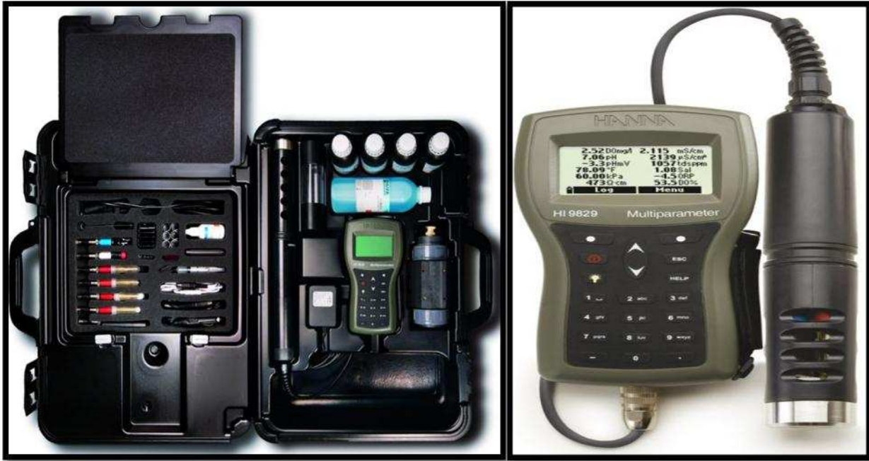
Figure 3.7 : HANNA Instruments HI 9829 multiparametre meter with available GPS, logging probe , turbidity, and ion measurement
