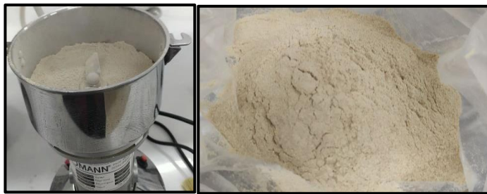
Figure 24 : Grinding and sieving of shrimp shells
