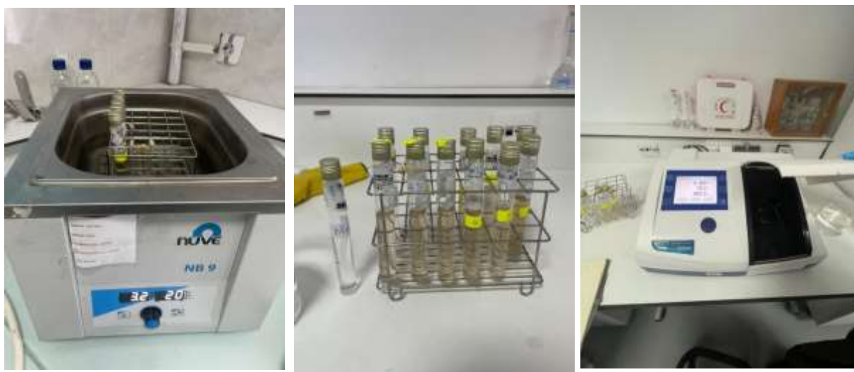
Figure 28 : Carbohydrate determination by the Dubois colorimetric method
