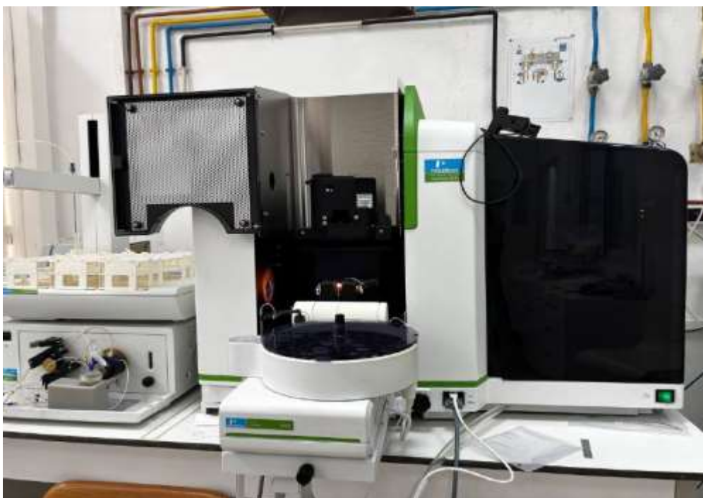
Figure 27 : Atomic Absorption Spectrometer (PerkinElmer PinAAcle™ 900H) used for trace metal analysis.
