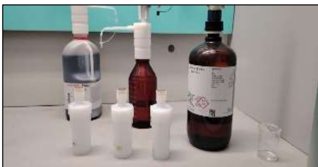
Figure 25 : Blank mineralization process with Teflon containers and acid treatment
