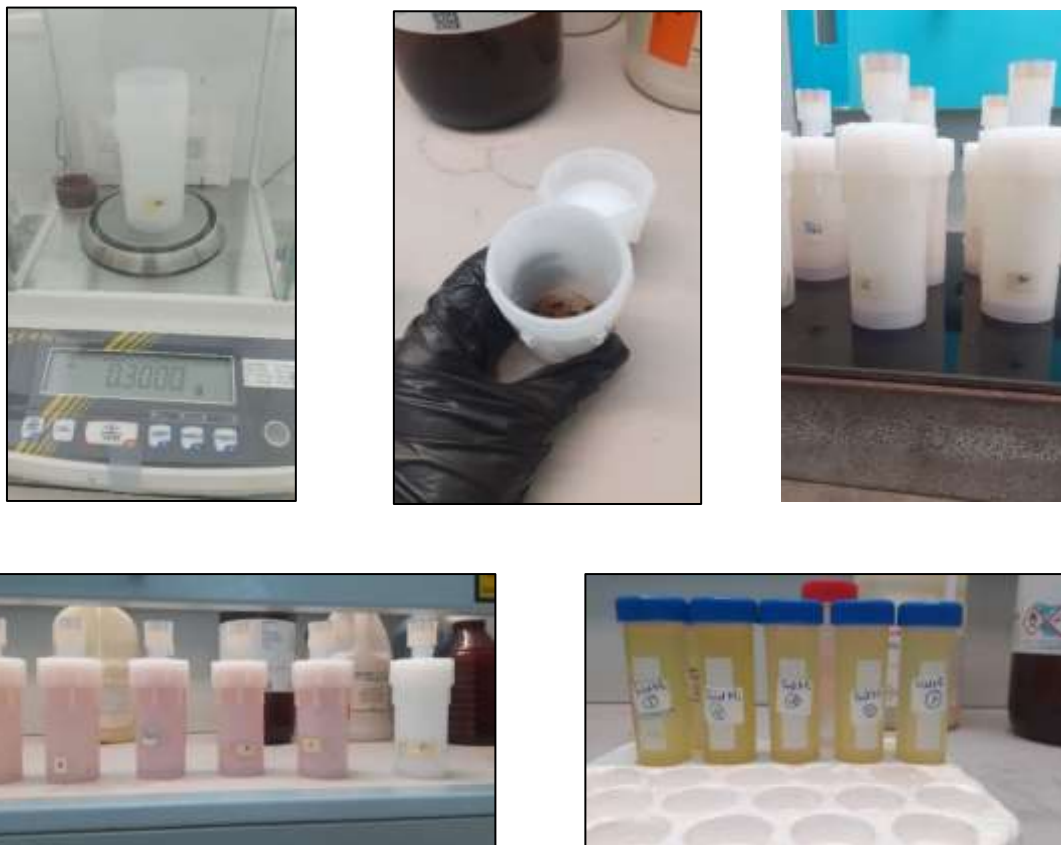
Figure 26 : Sequential steps of sample mineralization from sample weighing to final solutions before and after dilution.
