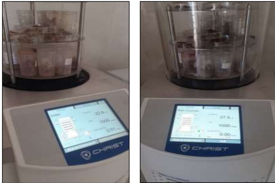
Figure 23: Lyophilization process using the Christ Alpha 1–2 LSCbasic freeze-dryer
