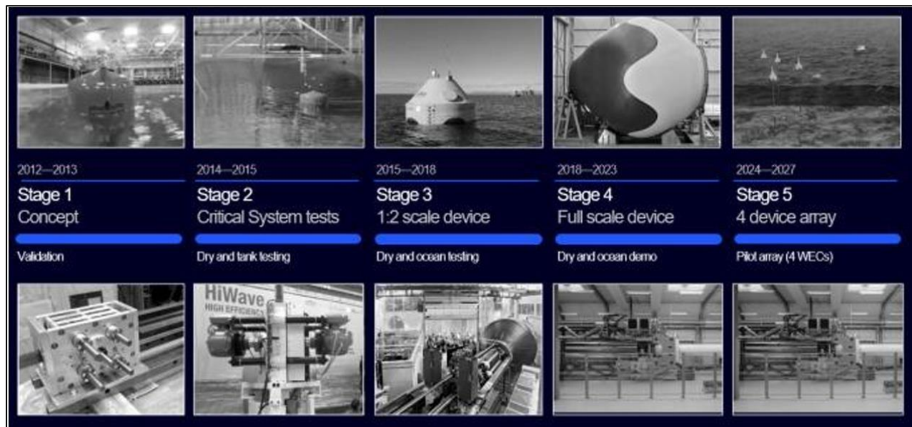
Figure 68: CorPower Ocean's Five-Stage Technology Verification Roadmap (2012–2027).
