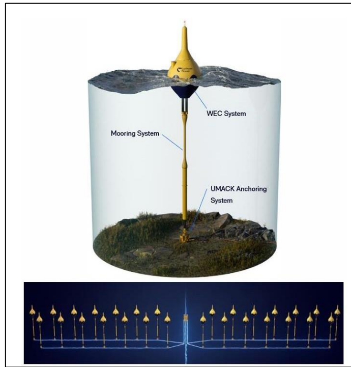
Figure 67 : CorPower Ocean C4 Mooring and Anchoring System.source,(Dickson et al., 2025)
