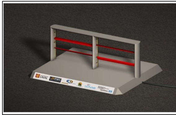
Figure 6: Conceptual configuration of an oscillating-foil hydrokinetic turbine (HAO). From: https://doi.org/10.1016/j.oceaneng.2015.05.011
