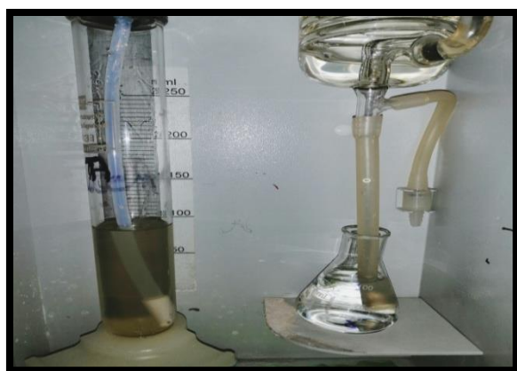
Figure II .6 : Distillation de l'ammoniac.
