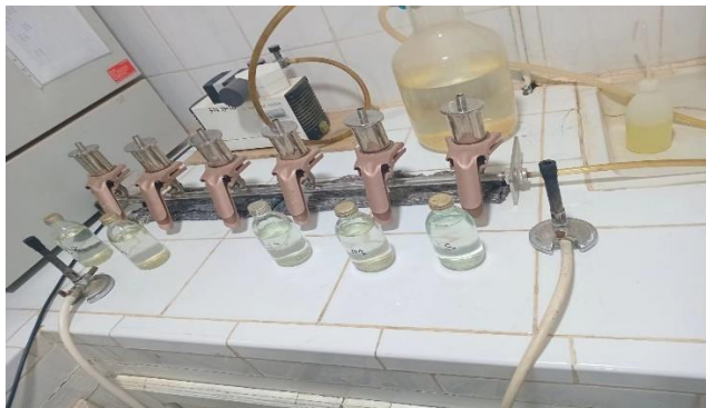
FIGURE 7: RAMPE DE FILTRATION
