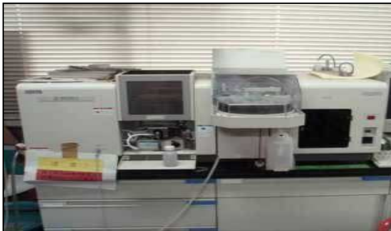
Figure II.16. SAA model HITACHI Z-5000
