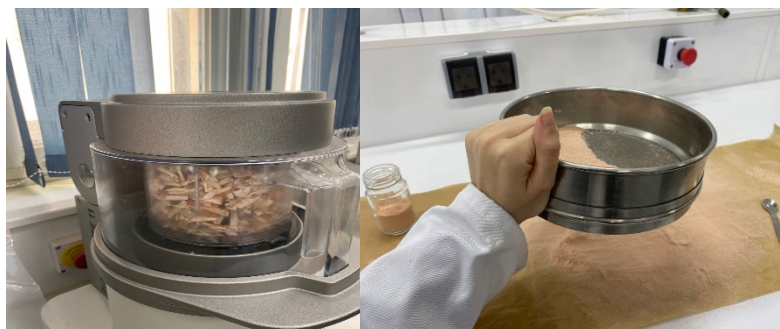
Figure 22: Broyage et tamisage
