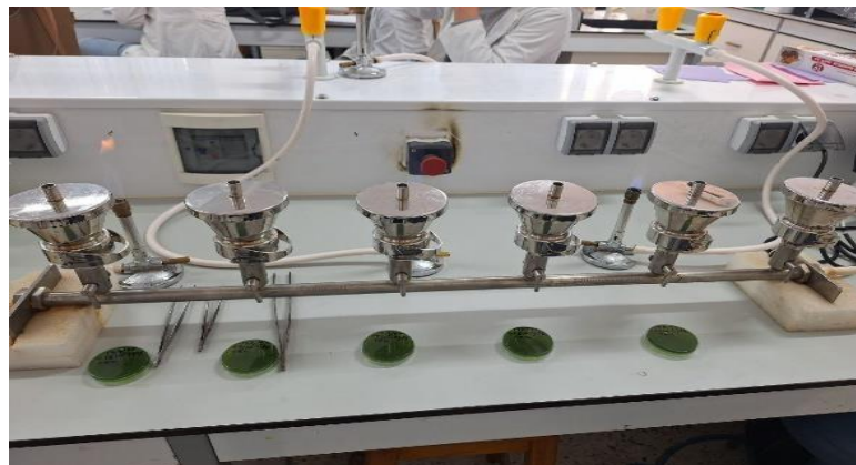
Figure 6: Rampe de Filtration
