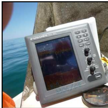
Figure II.2: Echosondeur de type FURUNO LS-4100.
