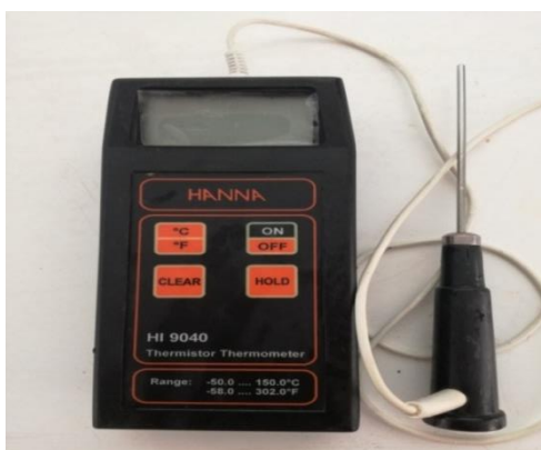
Figure II.13: Thermomètre (type HANNA HI 9040 )
