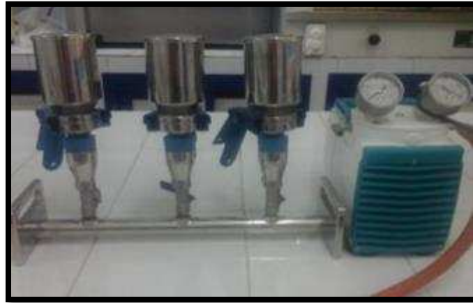
Figure III.7: Dispositif de filtration.
