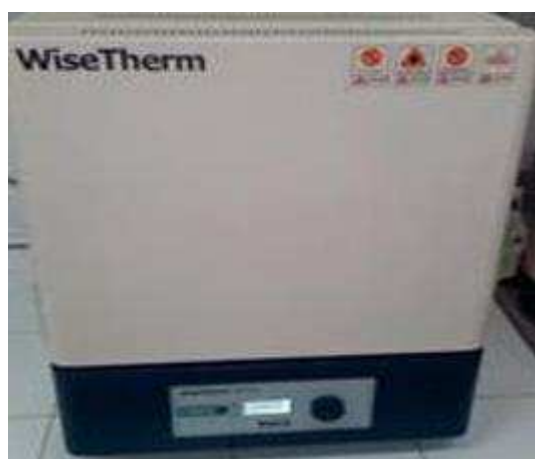
Figure III.8: Four à moufle (WiseTherm).
