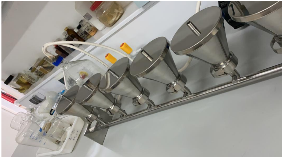
Figure 23 : Rampe a filtration
