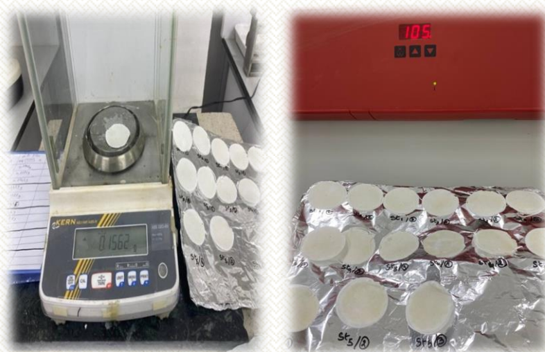
Figure II.9. Filter drying in the oven at 105°C and final gravimetric mass determination
