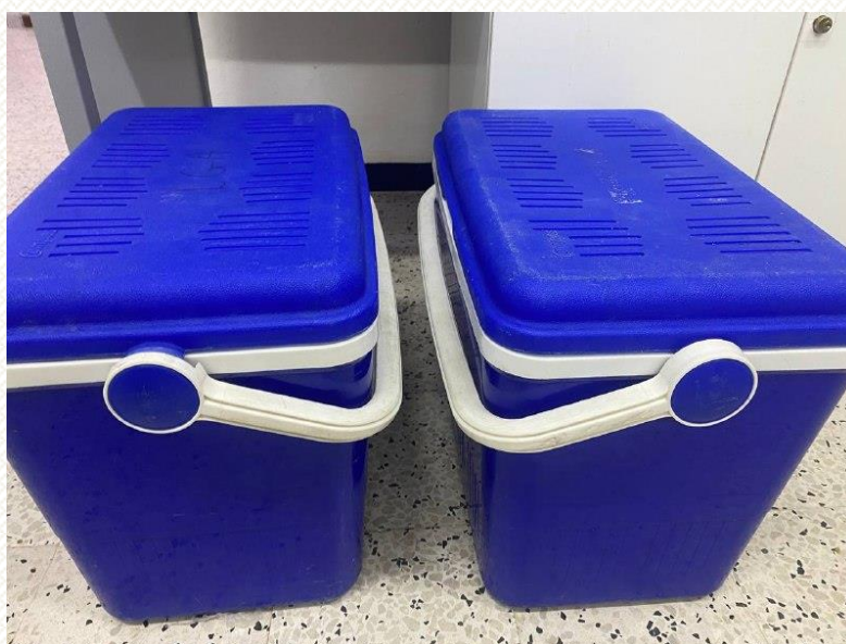
Figure II.7. Insulated iceboxes used for sample preservation and transport
