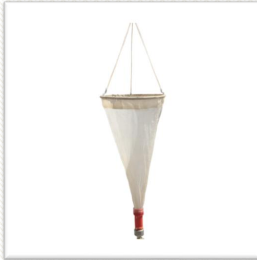
Figure II.5. A plankton net size of 20 \mu\text{m} .
