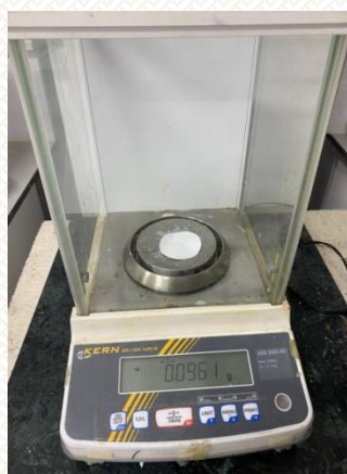
Figure II.8. Gravimetric filtration apparatus and analytical balance for TSS pre-weighing
