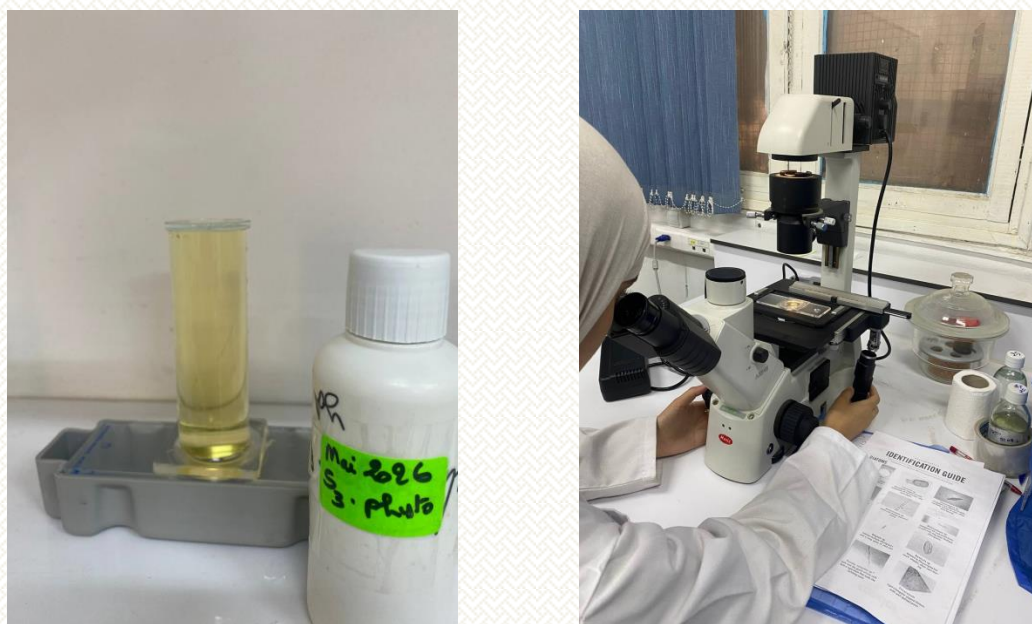
Figure II.10. Inverted microscope workspace and Utermöhl sedimentation chamber setup
