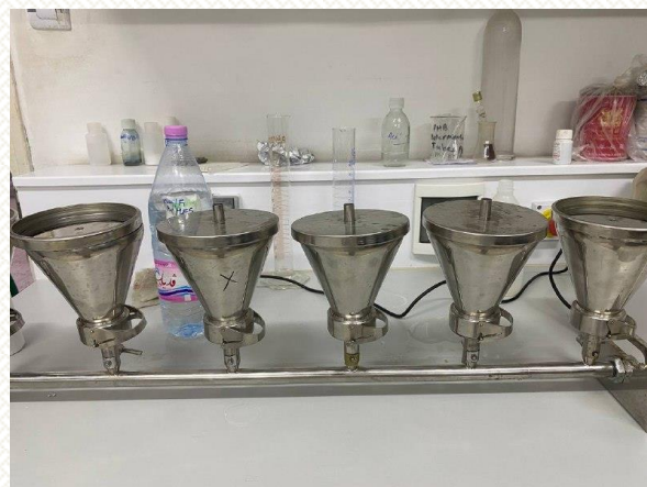
Figure II.8. Gravimetric filtration apparatus and analytical balance for TSS pre-weighing
