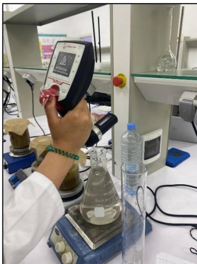
Figure 24: Verification of NaCl solution density using a densimeter
