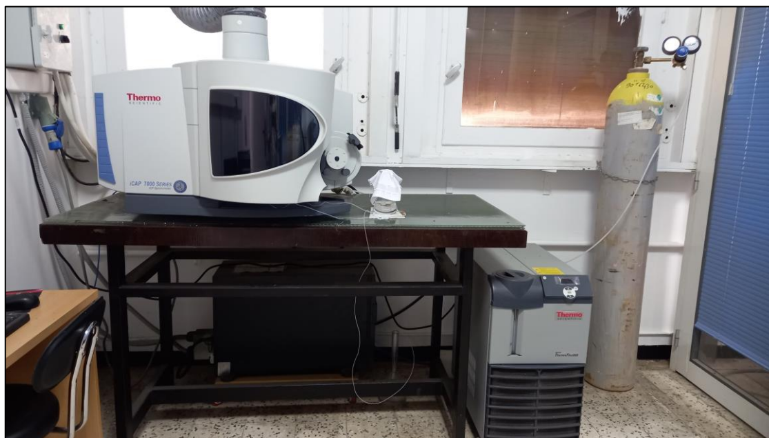
Figure 34: ICP-OES system used for trace metal analysis at CRNA laboratory
