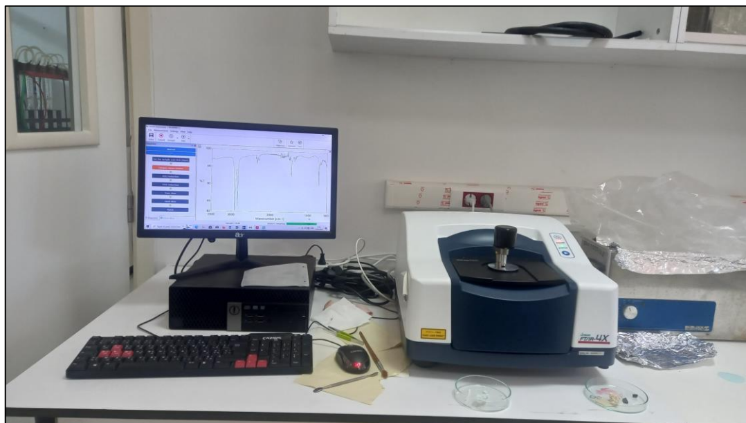
Figure 28: FTIR spectroscopy system used for the chemical characterization of MPs
