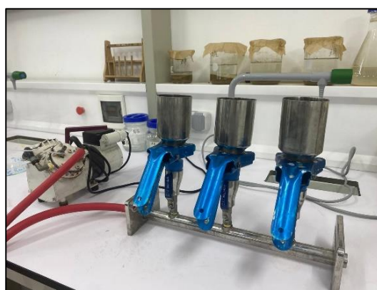
Figure 26: Vacuum filtration of the supernatant through GF/C glass fiber filters (1.2 \mu\text{m} )
